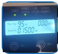
Real time O2 purity monitor
